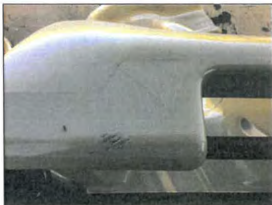
5. Cracked and sharp edges on slide hood
